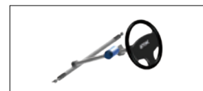
EPS steer by wire • Steering angle sensor
